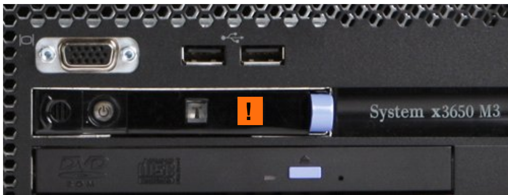
Front of Light Path Diagnostics Panel Amber light indicates there is a problem with the server
