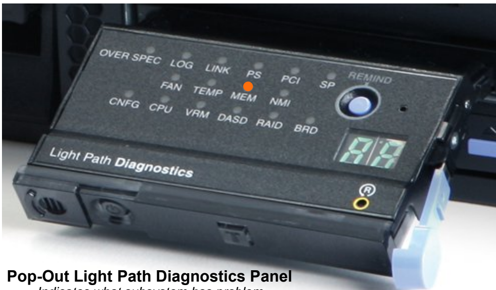
Front of Light Path Diagnostics Panel Amber light indicates there is a problem with the server
